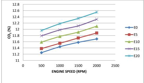
Graph 4.5 Variation of carbon dioxide and engine speeds for different blending ratios
