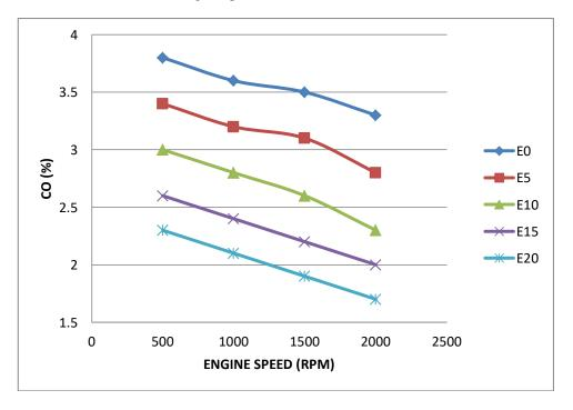
Graph 4.4 Variation of carbon monoxide and engine speeds for different blending ratios
