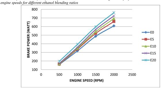
Graph 4.2 Variation of brake power and engine speeds for different blending ratios
